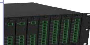
Various splitter modules in LGX Chassis
