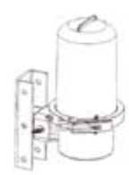
Vertical Mounting Position (Mounted To Cable Bearer)
