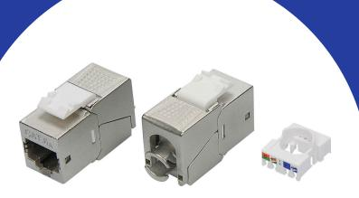
This series keystone jacks work together with high speed cables, cords and panels to provide performance beyond proposed Category 6A standards, a new feature of this series jack is a universal colored wiring label that eliminates the need for separate codes for T568A/B wiring scheme.
